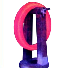
整体锻造法兰坯 integral forged flange bouble
